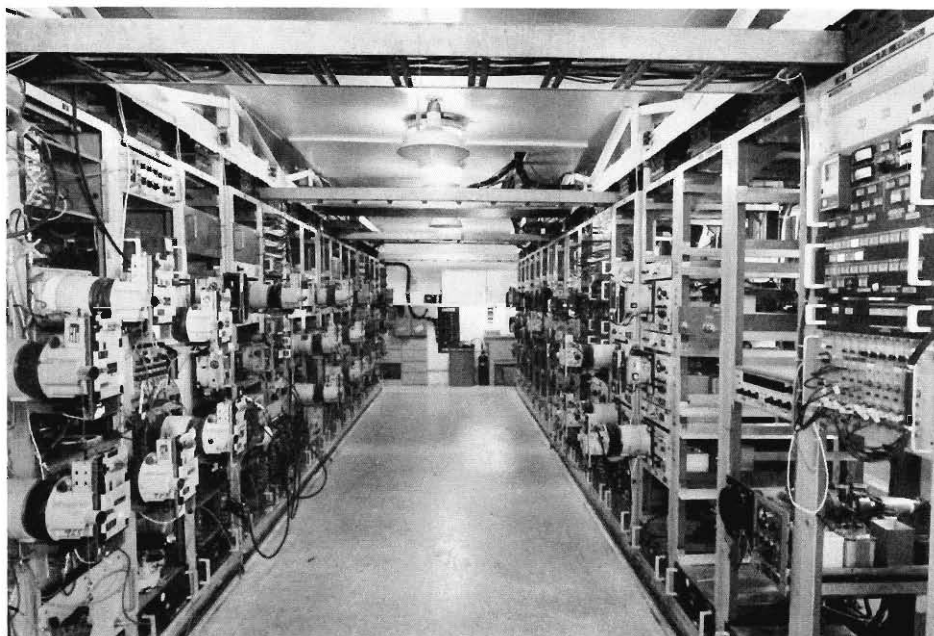
Interior of a diagnostics recording station with oscilloscopes and cameras.
