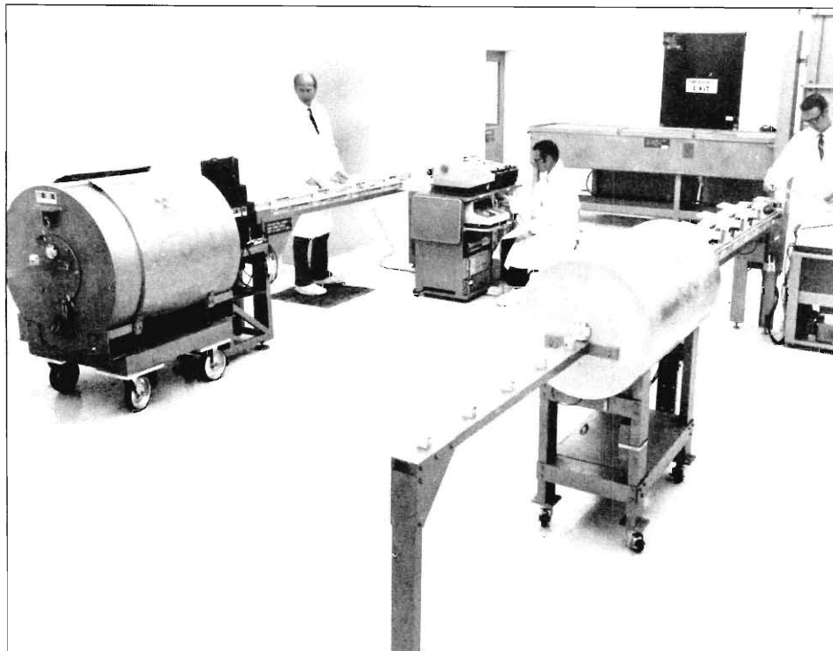
Nondestructive assay of fast breeder reactor fuel. Two fuel-rod scanners developed by Los Alamos are being used here in 1974 at the Hanford Engineering Development Laboratory as part of their safeguards and quality control. The device on the left uses a computerized californium-252 system to measure both plutonium content with an accuracy of better than 0.5 percent and pellet-to-pellet uniformity of fissile material loaded into the rod. The system on the right uses a passive neutron-coincidence technique to measure plutonium-240 content, thus providing a cross-check with the first instrument.
